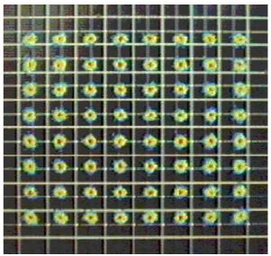
64 QAM signal with signal I/Q amplitude error of the converter
